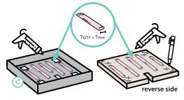
Ensure the adhesive supports each corner OF THE INLAY MATERIAL above and below the Height Adjuster.
