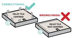
Make sure the glue has stiffened and remains flush with the inlay cover.
