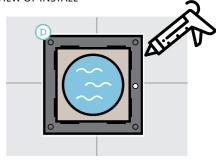
The Edge Protector may be left loose on its mortar bed or filled with an expansion joint gap filler to allow for expansion and contraction of the steel.
